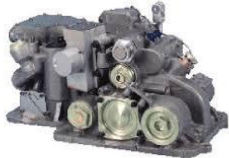
Gambar 1 Housing Valve Propeller Control C 130 Hercules
