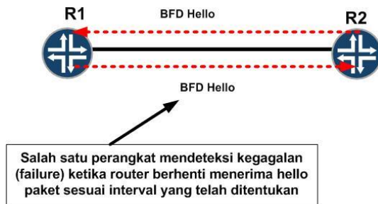
Gambar 2. Sistem kerja BFD ( Bidirectional Forwarding Detection )
