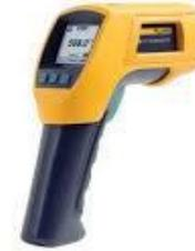
Gambar 6 Thermometer digital fluke
