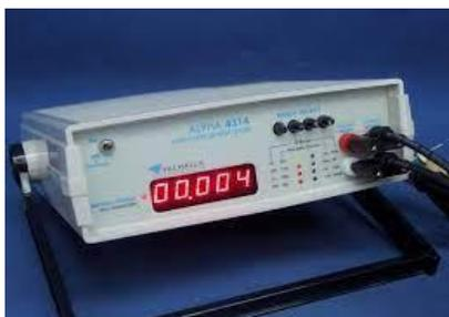
Gambar 5 Igniter tester Alpha 4314
