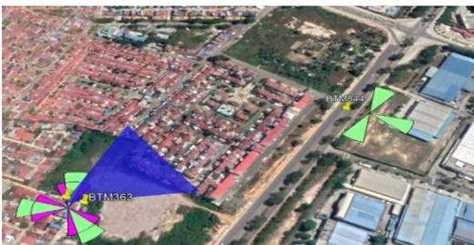
Gambar 10. Simulasi *lower Coverage* Gnet Tilt Setelah
