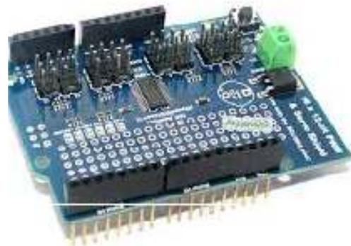
Gambar 5. servo shield 16-Channel 12-bit PWM
