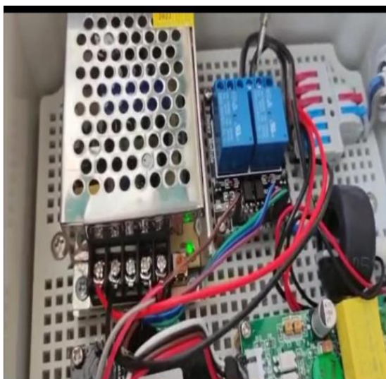
Gambar 7. Alat Monitoring Daya Pintar
